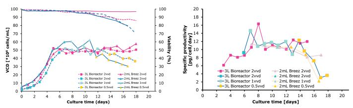
Overall, the data shows broad comparability between the Mobius® Breez Microbioreactor and the 3 L benchtop reactor, indicating Mobius® Breez is a suitable scale-down model for perfusion performance predictability. The data also showcases the benefits of running perfusion, which allows for several experiments to be performed in the same run, thus saving time. In this instance, the experiment shifted from 2 vvd to 1 vvd on day 8 and then to 0.5 vvd on day 12.
